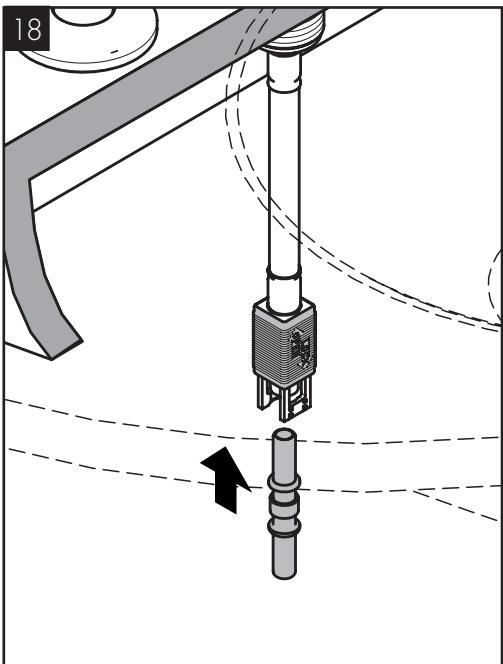
Insert the connector into the quick connect.
