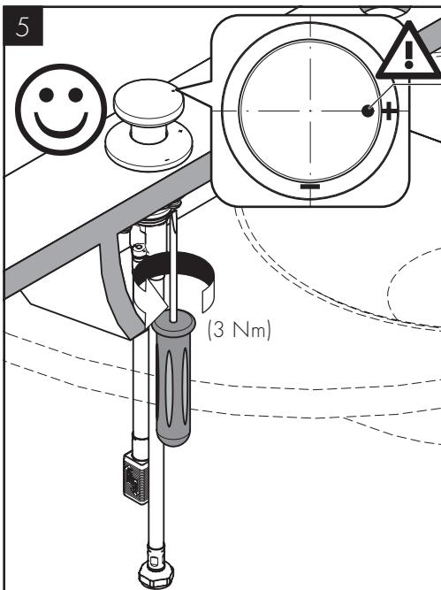
Tighten the mounting nut. Tighten the tensioning screws.
