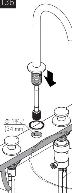
If the hole on the mounting surface is 34 mm, install the spout without the sealing ring.
