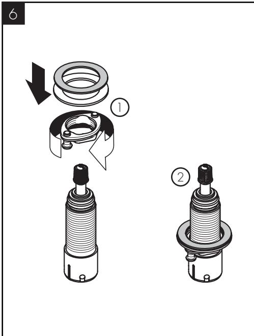
Install the mounting nut, metal washer, and fiber washer on the adapter assembly.
