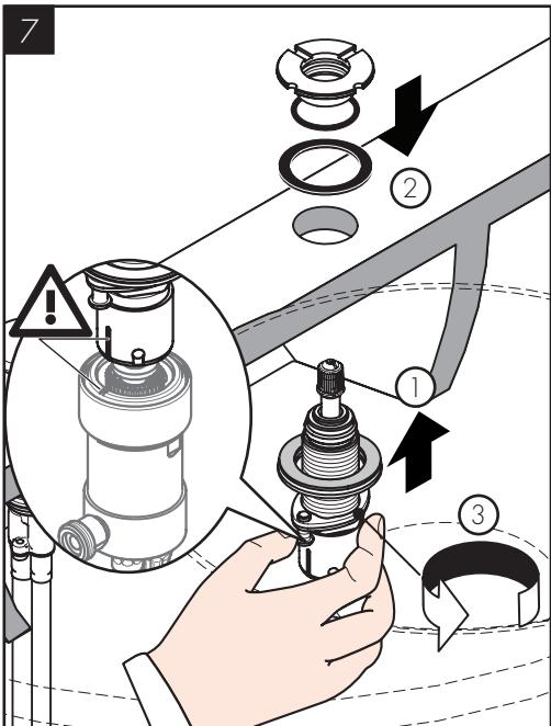
Push the adapter assembly up through the mounting surface. Install the holder, the o-ring, and the seal. Rest the holder on the mounting surface.
