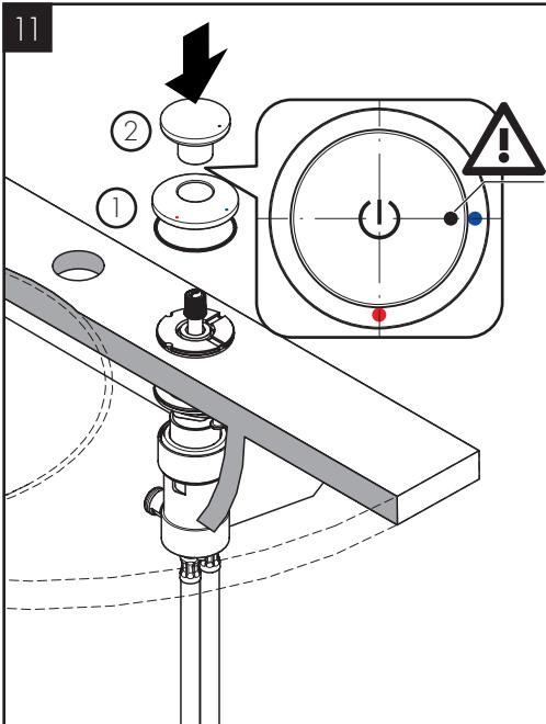
Install the escutcheon and O-ring on the holder. The blue dot must be on the right and the red dot at the front.
