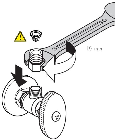
Install the adapters on the stops.
