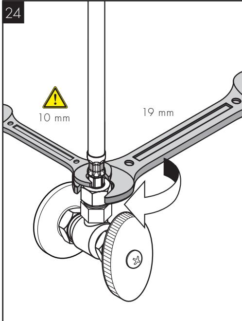
Connect the hoses to the stops using two wrenches.
