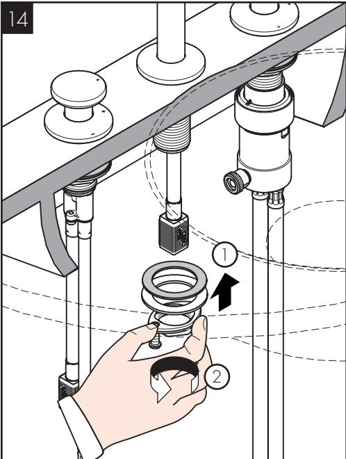
Install the fiber washer, the metal washer, and the mounting nut.
