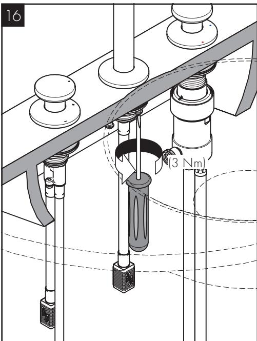
Tighten the mounting nut.
