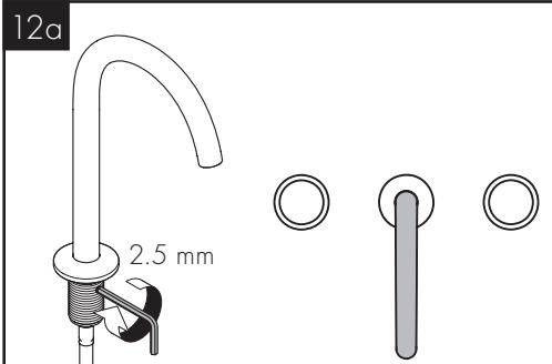
If the homeowner wishes the spout to be fixed in one position, tighten the set screw on the front of the shank using a 2.5 mm Allen wrench.
