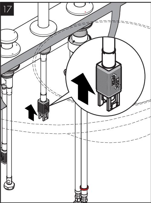
Open the quick connect on the spout hose by pushing it upward.
