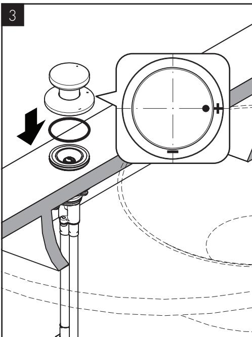
Align the dot on the handle with the “+” sign on the escutcheon. The “-” sign on the escutcheon should be at the front, the “+” sign should be at the right.
