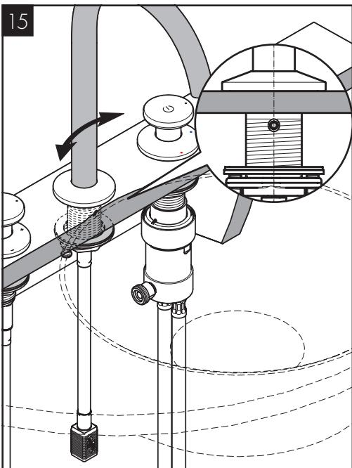
Pivot the spout if necessary. The set screw should be at the front.
