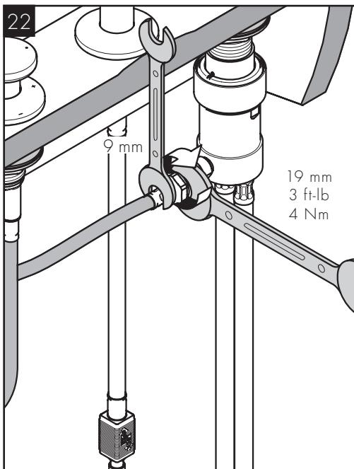
Connect the volume control connection hose to the function block.
