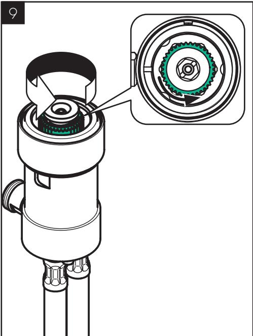
Rotate the function block valve stem counterclockwise as far as it will go without using force.
