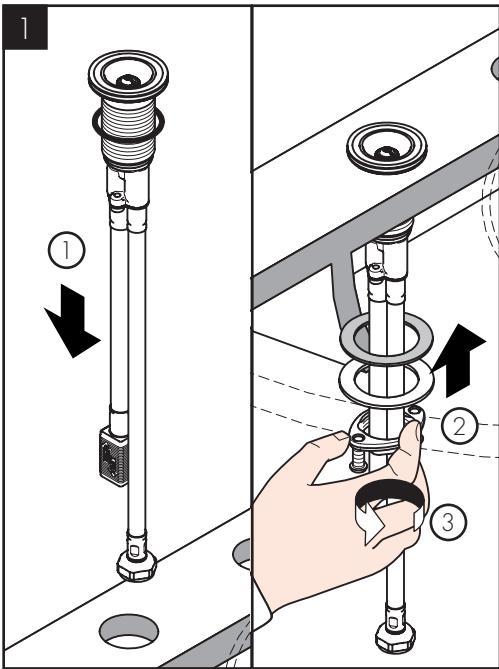
Place the volume control assembly on the mounting surface.
