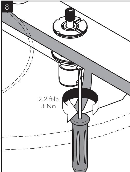
Tighten the mounting nut.
