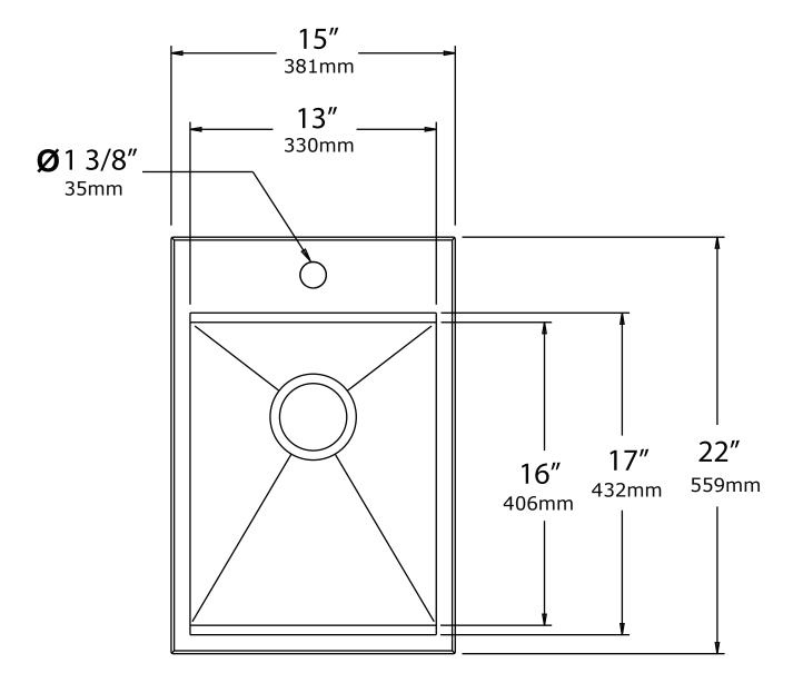
**NOTE:** Cutout template is provided as a guide **ONLY** and must be checked against actual sink to verify correct fit.
