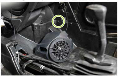
b. Position the speaker in place. Refasten the T40 Torx screw through the bracket pre-attached to the bottom of the speaker.
