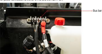
Remove the top dash panel and upper storage compartment to access the dash cavity for installation of the BPS1RS and RZR-FSA.
