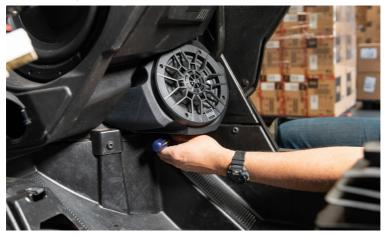
c. Using two of the supplied screws (M5x27mm), secure the speaker to the firewall via the other two mounting holes on the speaker. Install the left/amplified speaker near the footwell on the driver side. Repeat the right speaker installation steps to the driver side.
