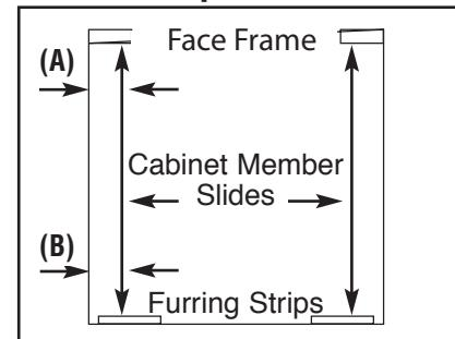
**Step 5:** Mount Rear Bracket. Extend the slide rear mounting bracket until it contacts the rear (Furring Strip). Bottom of slide should be  $14\frac{1}{2}$ " from cabinet floor. Rear mounting bracket should be the same distance from the side cabinet wall at rear of slide as it is up front. Drive mounting screw in center horizontal slot of rear mounting bracket, tighten. Tighten screw in front bracket.
