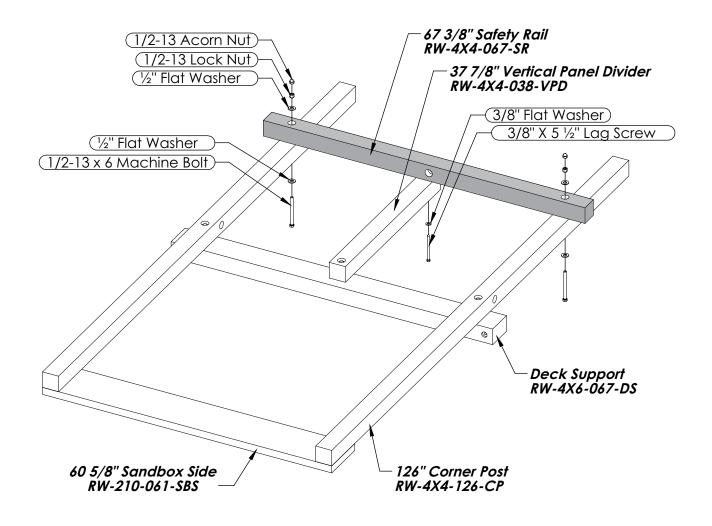
3. While flat on the ground lay Corner Posts parallel on the ground and attach Deck Support and Sandbox Side as shown.
