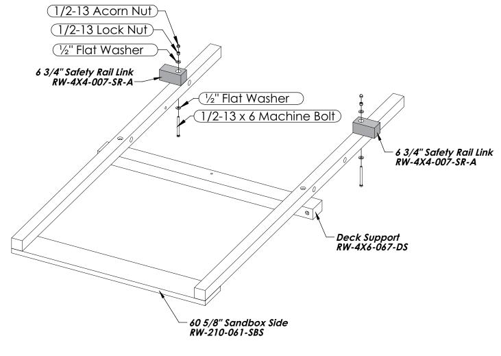
5. Attach Safety Rail, Deck Frame and Sandbox Side as shown.
