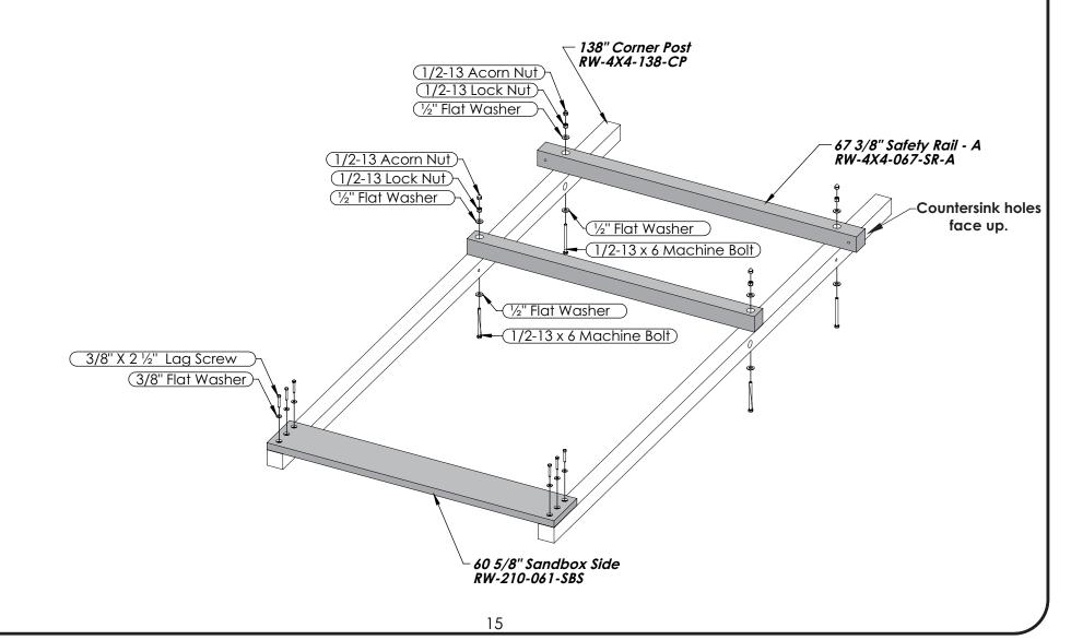
20. Assemble Safety Rails and Deck Supports to Corner Posts as shown. Do not install 74 1/8" Safety Rail Right RW-4X4-074-SR-R Lag Screws until indicated. 74 1/8" Safety Rail Left RW-4X4-074-SR-L 74 1/8" Deck Support Right RW-4X6-074-DS-R 74 1/8" Deck Support Left RW-4X6-074-DS-R¬ 1/2-13 x 6 Machine Bolt (½" Flat Washer 1/2" Flat Washer (1/2-13 x 6 Machine Bolt) (1/2-13 Lock Nut) (1/2-13 Acorn Nut) Countersink holesface down 1/2-13 Acorn Nut (1/2-13 Lock Nut) ½" Flat Washer
