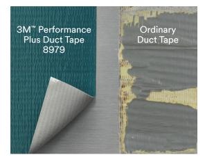
3M™ Performance Plus Duct Tape 8979 holds up to weathering exposure and removes cleanly.
