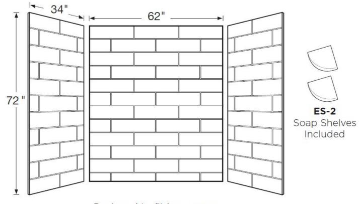
Designed to fit base areas 34" deep or smaller x 62" wide x 72" high or smaller (864 mm x 1575 mm x 1829 mm)
