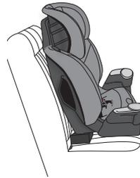
Place the foam block on the center of a vehicle seat making sure it is pushed up against the vehicle seat back. Place the rear of the booster seat centered on the foam block. Follow all the other instructions in this owner's manual.
