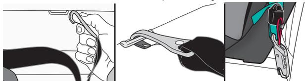
Refer to your vehicle owner's manual to locate the lower anchor bars on your vehicle seat. Attach the right hook, or clip, to the right anchor bar and the left hook, or clip, to the left anchor bar. Double check that the lower anchor connector hook is fully engaged by pulling hard on the lower anchor connector strap. Make sure vehicle seat belt lies flat without twisting.
