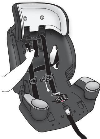
4. Route the harness straps through adjustment slots, then attach to splitter plate.
