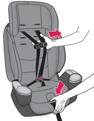
**2. Remove both harness straps from the splitter plate and pull them through to the front of the seat.**
