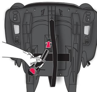
Insert the crotch strap anchor back into the opening from the bottom of the child restraint.
