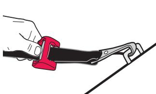
Press the adjuster release button to loosen.
