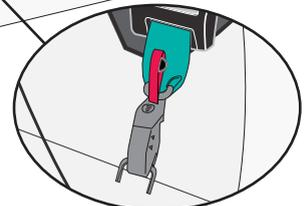
To remove the hook, press the tab and twist, then remove from anchor.
