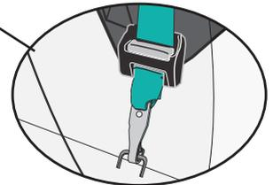
Tilt and slide the adjuster to loosen.
