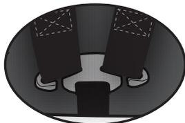
Make sure both harness straps are installed **completely** on the splitter plate, as shown.
