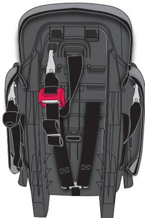
Disconnect from the back of the child restraint.
