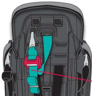
1. **Disconnect tether hook from the back of the child restraint.**
