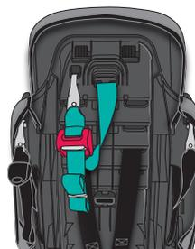
1. **Disconnect tether hook and lower anchor connectors from the back of the child restraint.**
