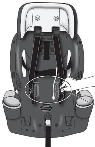
5. Fold and tuck the harness, chest clip and buckle tongues into the recesses on either side of the seat shell.
