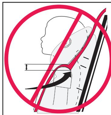
**IMPORTANT:** If the child's shoulders are high enough that routing the shoulder belt under the head rest causes the belt to be pulled down the back side of the child's shoulder (before passing through the head rest) the belt should not be routed between the seat and the head rest.
