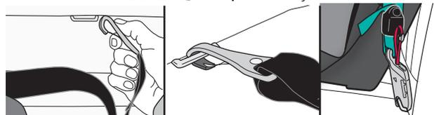
Refer to your vehicle owner's manual to locate the lower anchor bars on your vehicle seat. Attach the right hook, or clip, to the right anchor bar and the left hook, or clip, to the left anchor bar. Double check that the lower anchor connector hook is fully engaged by pulling hard on the lower anchor connector strap. Make sure vehicle seat belt lies flat without twisting.
