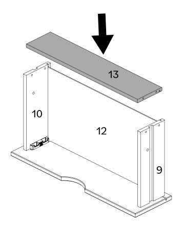
Secure the Drawer backs (13) inserting all Plastic screws (K) in the holes on the Right drawer sides (9) and Left drawer sides (10). Use a hammer if necessary.
