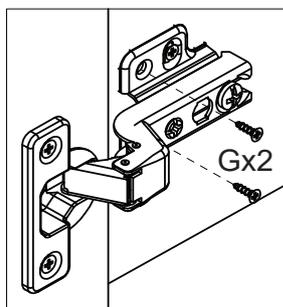
Once all the adjustments are complete and both doors are aligned, fix remaining x8 screws (G) into the other hinge plate holes then check all the other hinge screws are tight.
