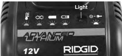
Figure 5 – Charger LED Light and Markings
