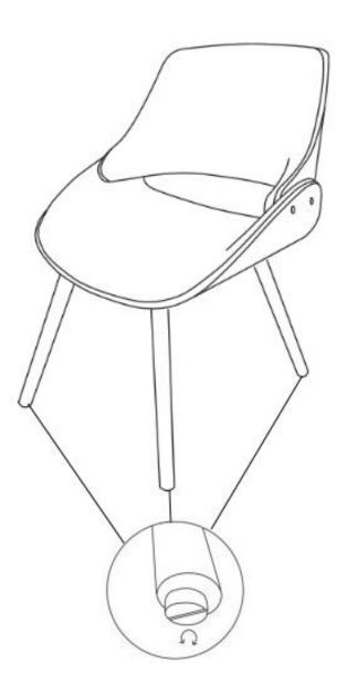
Place Chair on a flat level surface to ensure it is level. If it is uneven, adjust the leg levelers on the bottom of the legs.
