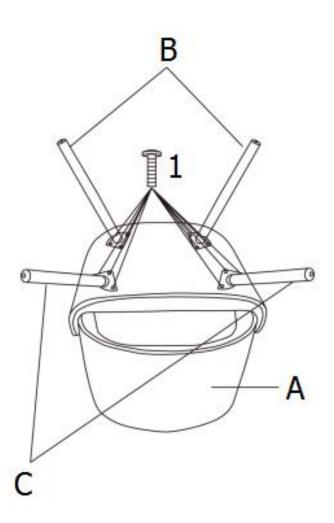
Attach the Front Legs (B) and Back Legs (C) to the Seat (A) with Allen Key Screws (1). Use Allen Key (2) to tighten.
