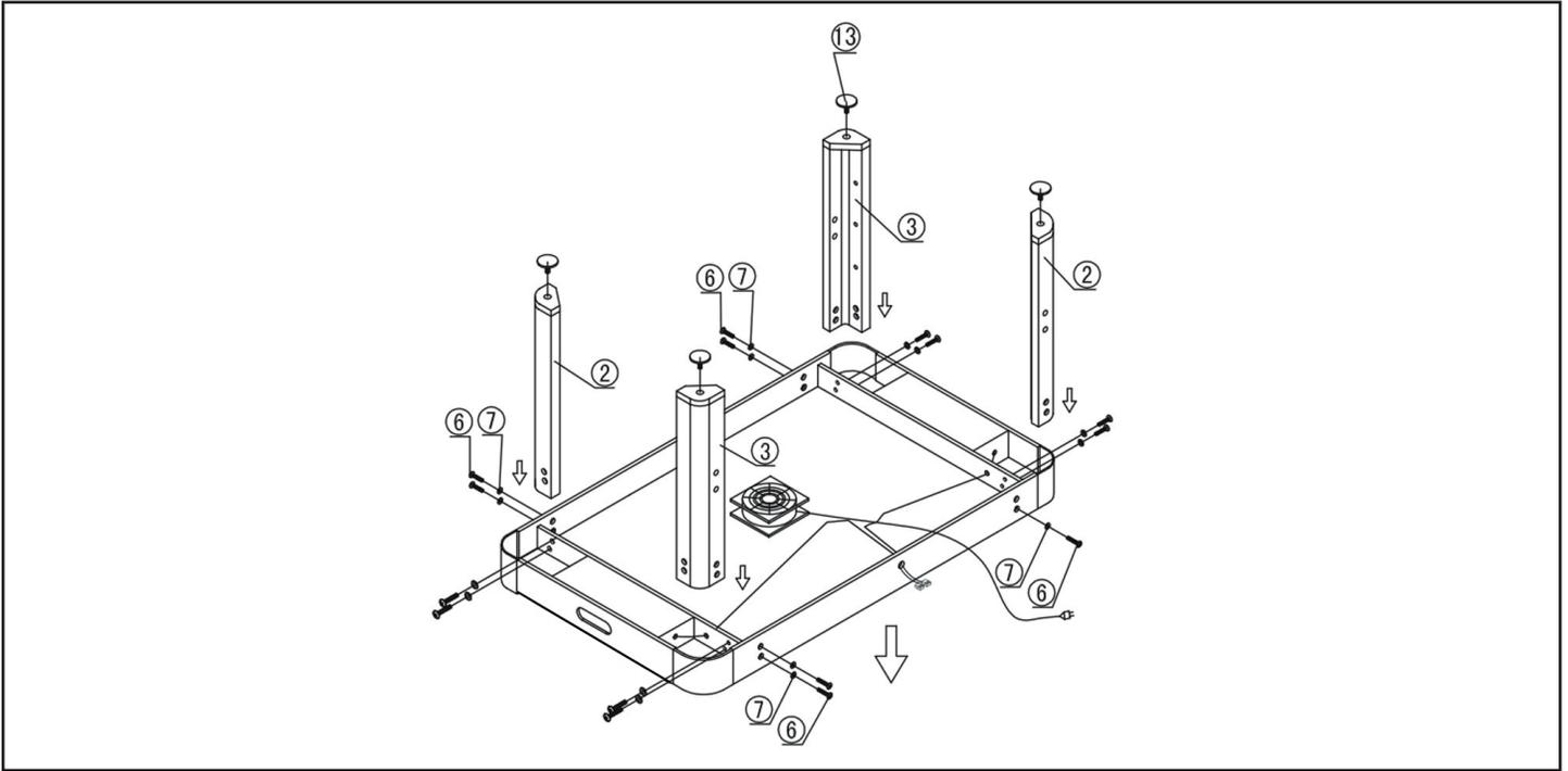
3. Attach each LEG PANEL #4 to LEGS as shown with SCREW #10. *Note: Graphics should face outward.*
