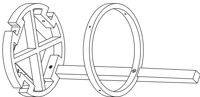
Do not tighten bolts completely until all bolts are completely lined up and inserted into holes.
