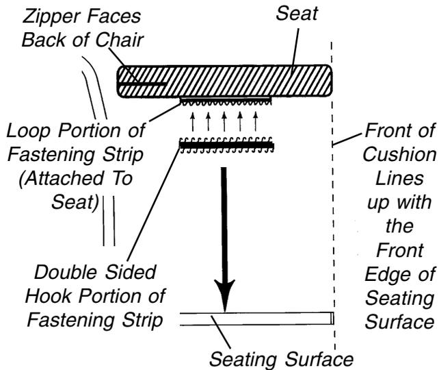
FIGURE 1- ATTACHING/ REMOVING
