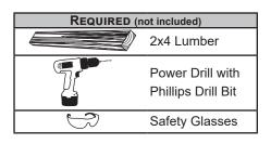
**NOTE:** Lumber not included. Lumber is nominal size and may need to be planed or sanded to fit inside the bracket slots.
