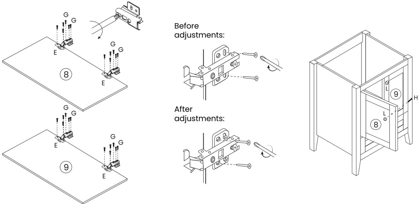
**Hinge/Door Adjustment and Realignment**
