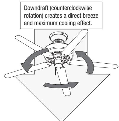
Downdraft (counterclockwise rotation) creates a direct breeze and maximum cooling effect.
