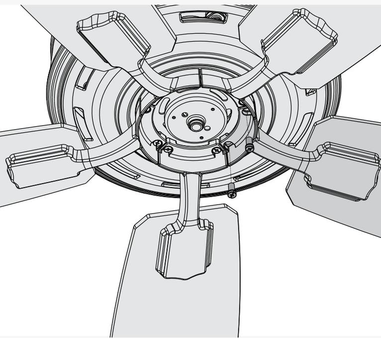
Lightly attach the blade arms to the motor with the blade arm screws, then securely tighten after both screws are attached.
