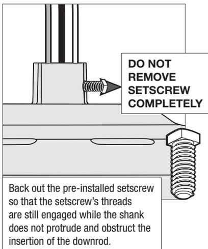
Back out the pre-installed setscrew so that the setscrew's threads are still engaged while the shank does not protrude and obstruct the insertion of the downrod.
