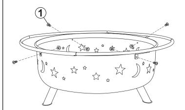
Carefully guide the assembled ring over the fire bowl and align the safety ring brackets with the fire bowl mounting holes. Then, loosely fasten the ring to the bowl using four M6x12mm Bolts (1) and M6 Nuts (2).
