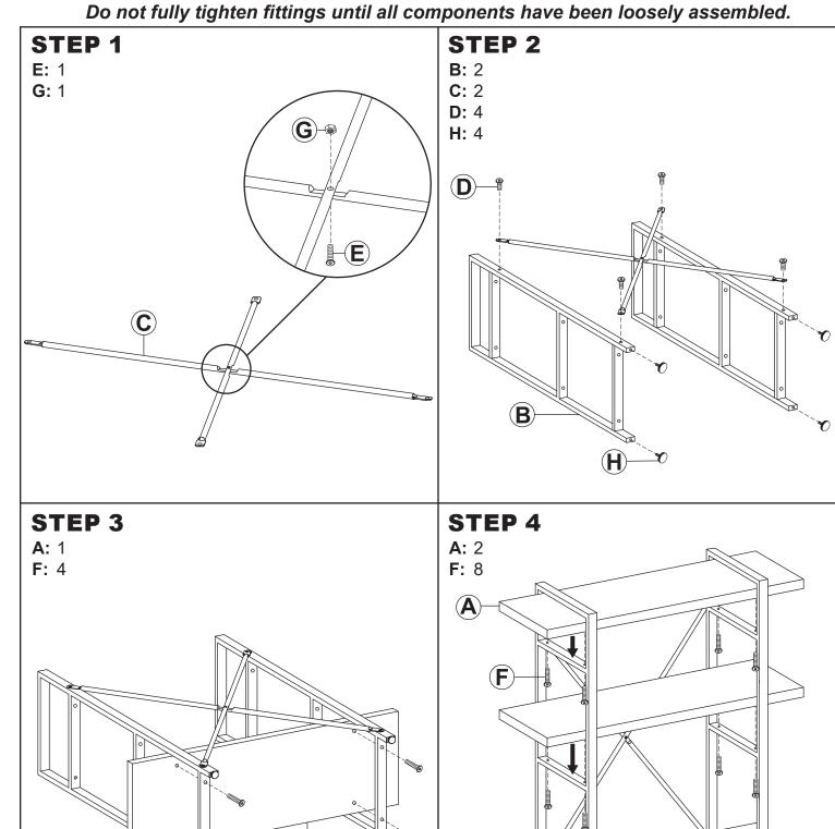
Tighten all fittings; do not over-tighten.
