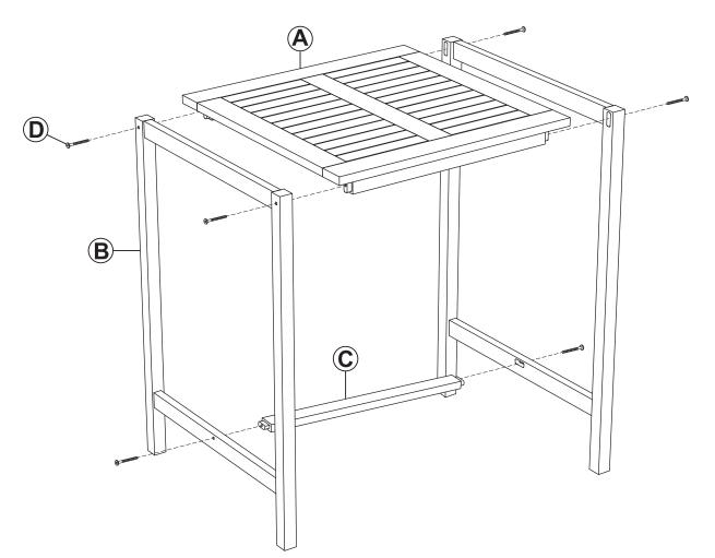
Align Tabletop (A) with one Leg Panel (B) and loosely securing using two M6x5cm Bolts (D).
