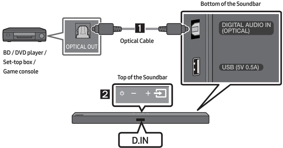
1. Connect **DIGITAL AUDIO IN (OPTICAL)** on the main unit to the **OPTICAL OUT** jack of the Source Device using a digital optical cable.
