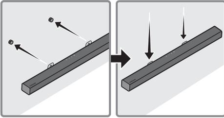
8. Slide the Soundbar down as shown below so that the **Bracket-Wall Mounts** rest securely on the **Holder-Screws**.
