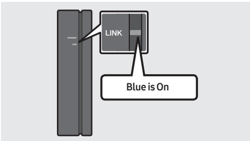
The LINK LED indicator stops blinking and glows a solid blue when a connection is established between the Soundbar and the Wireless Receiver Module.
