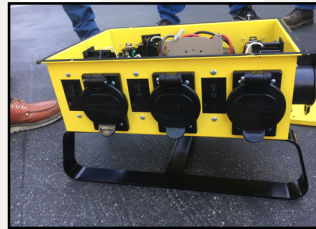
Image A is a Southwire Box with thicker gauge metal and a center support bar.
