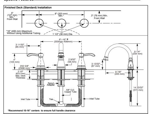
Rough Deck (Thick Tile) Installation 5" (127 mm) Min.\* From Wall 8" (203 mm) Min \* ' (76 mm) Min. From Wall \*16" (406 mm) Maximum Without Using Additional Tubing 2" (51 mm) Dia 8"~16" **\*** mm~406mm) 3 11/32" (85 mm) 9 1/4" (234 mm) 2 9/32 4" (103 mm) (58 mm) 3 13/32' (87 mm) 2X2 5/8" (2X66 mm) 2 1/2" (63.5 mm) Max. Deck Thickness . 8 7/8" (225 mm) 5/8" O.D. Copper Tube 14 23/32 (373 mm) Inlet Tube Inlet Tube \*Recommend 10-16" centers to ensure full handle clearance
