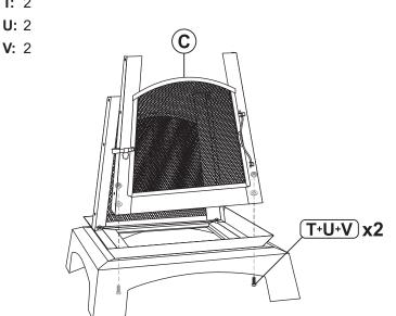
Fasten Front Screen (C) using two Bolts (T), Washers (U), and Nuts (V), as shown.
