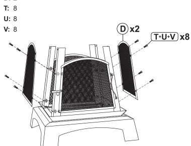
Secure each Side Screen (D) using four Bolts (T), Washers (U), and Nuts (V).
