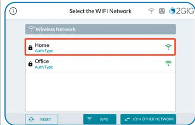
After the Keypad has connected to the chosen WiFi network, you'll be prompted to press PAIR on the Main Panel.
