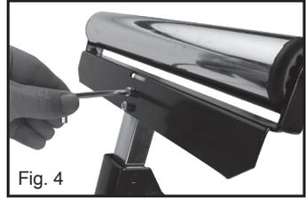
**NOTE:** Set the roller assembly parallel with a support stand or other saw table to better support longer work-pieces.
