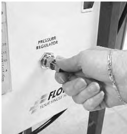
Pressure regulator valve on panel
