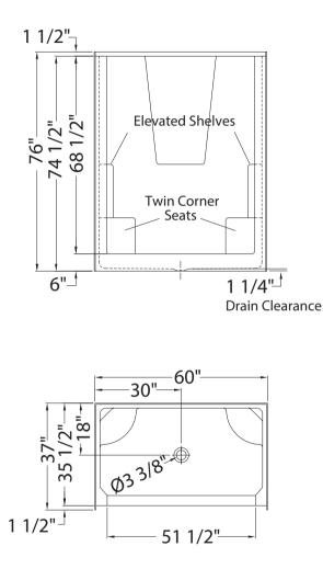
All dimensions are approximate. Structure measurements must be verified against the unit to ensure proper fit.
