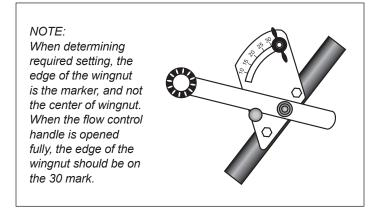
**IMPORTANT: REMEMBER TO START AND STOP THE SPREAD WHILE MOVING.** Do not open the flow control lever while stopped or material will simply run onto the ground without being spread.
