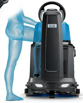
The lowered footboard facilitates easy access from both sides and allows the operator to sit comfortably.
