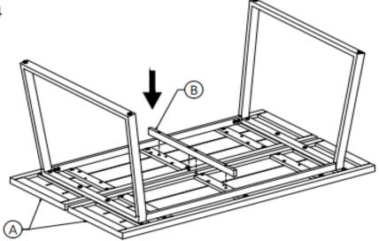
1. Attach Connector Bar (B) to Tops (A).
