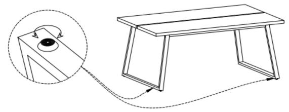
Note: Levelers on bottom of legs can be adjusted if floor is uneven.
