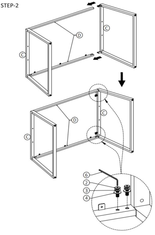
1. Repeat Step-1 to secure parts  $\bigcirc$  with the second Leg  $\bigcirc$ .
