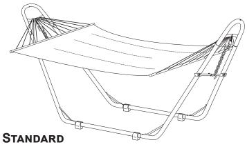
Hang standard-sized hammocks over the top frame crossbars. Use the S-hooks and chains to adjust the hammock height as needed.
