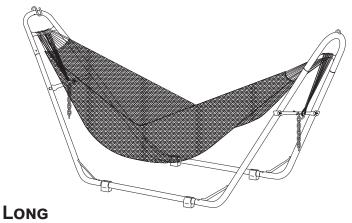
Drape the ropes of long hammocks over the top frame crossbars and secure the ends to the hook bolts.
