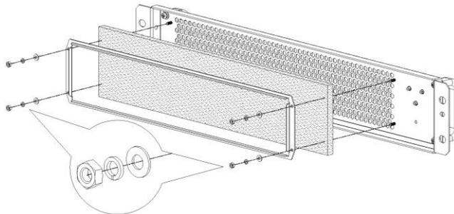
4. Install the front cover and lock the screws.
