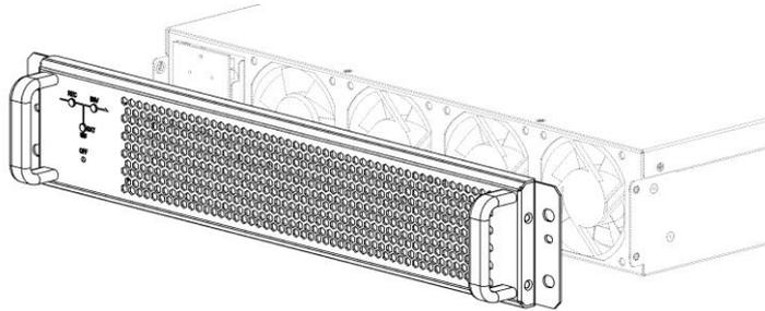
3. First Installation: Install the sponge board, sheet metal, washers and nuts.
