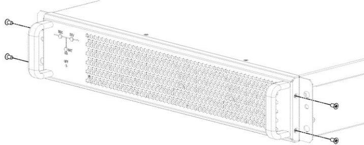
2. Remove the front cover from power module.
