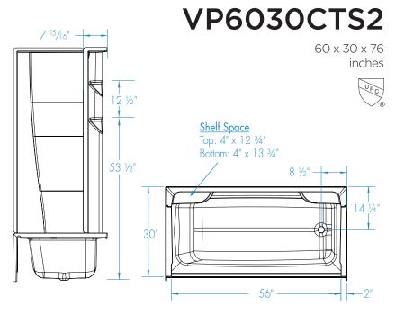
FEATURES Dimensional Tolerance ± 3/8". Dimensions needed for site preparation should be measured from the unit. Manufacturer assumes no responsibility for preparatory work.
