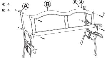
Fasten Backrest (B) to Arm Panels (A) using M6x30mm Bolts (1), Washers (4), and Nuts (6).
