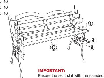
Fasten Seat Slates (C) to the arm panels using M6x30mm Bolts (1), Washers (4), and Nuts (6).
