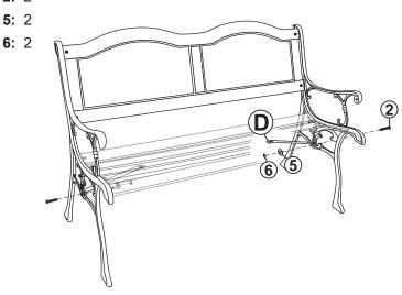
Attach Side Braces (D) to the arm panels using M6x20mm Bolts (2), Washers (5), and Nuts (6).
