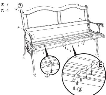
Secure the side braces to the seat using M3x15mm Scews (3).
