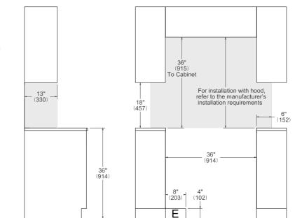
NOTE a. Electrical Connection b. Gas Connection
