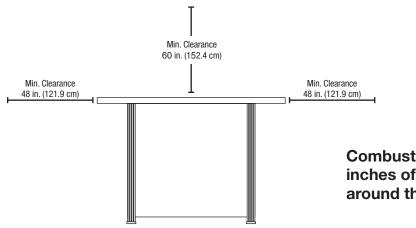
Combustible materials should not be within 60 inches of the top of the unit, or within 48 inches around the entire unit.
