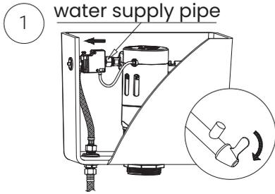
Shut off the water supply valve, then remove the water supply pipe.
