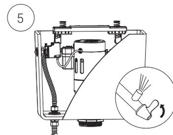
Insert the water supply pipe back to the water connector and turn on the water supply valve.
