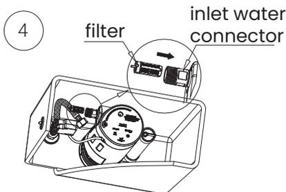
Re-install clean filter back into water connector.
