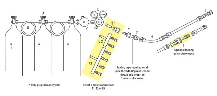
Note: DO NOT use teflon sealing tape on straight threaded connections with O-ring seals.
