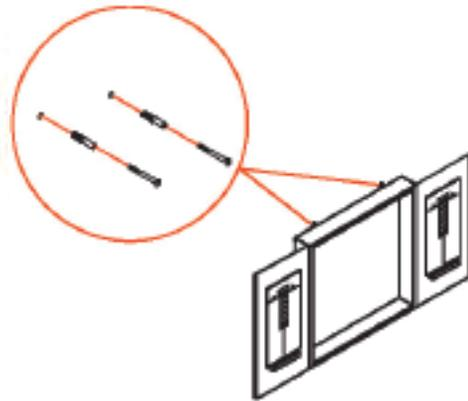
Step 2: Select a drill bit that is roughly the same diameter as the Plastic Anchors (#5) included in the hardware package. Once the holes have been drilled, use a hammer and tap the Plastic Anchors (#5) into the hole. Once the Plastic Anchors (#5) have been inserted, you may screw the 1.3" Screws (#2) into them.
