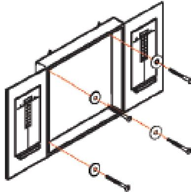
Step 2: Once you are certain the marks are at the proper height and they are located at the wood studs, have someone hold the Dartboard Cabinet (without the **Bristle Dartboard (#1)**) against the wall. Make sure that the four holes in the Cabinet are lined up with your previous pencil marks. Now use an electric screwdriver to screw the **2" Screws (#3)** with **Washers (#4)** directly into the wall making sure to drill into the wood studs.
