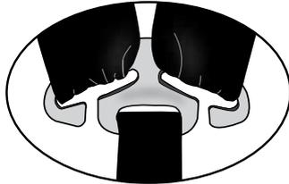
**IMPORTANT:** Make sure both harness straps are installed **completely** on the splitter plate, as shown.
