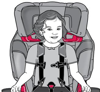
**Note:** Straps must be positioned at the child's shoulder level or slightly above. Harness Covers **MUST** be installed when using the 5-point harness for children weighing 18 kg (40 lbs) or less (see page 54).
