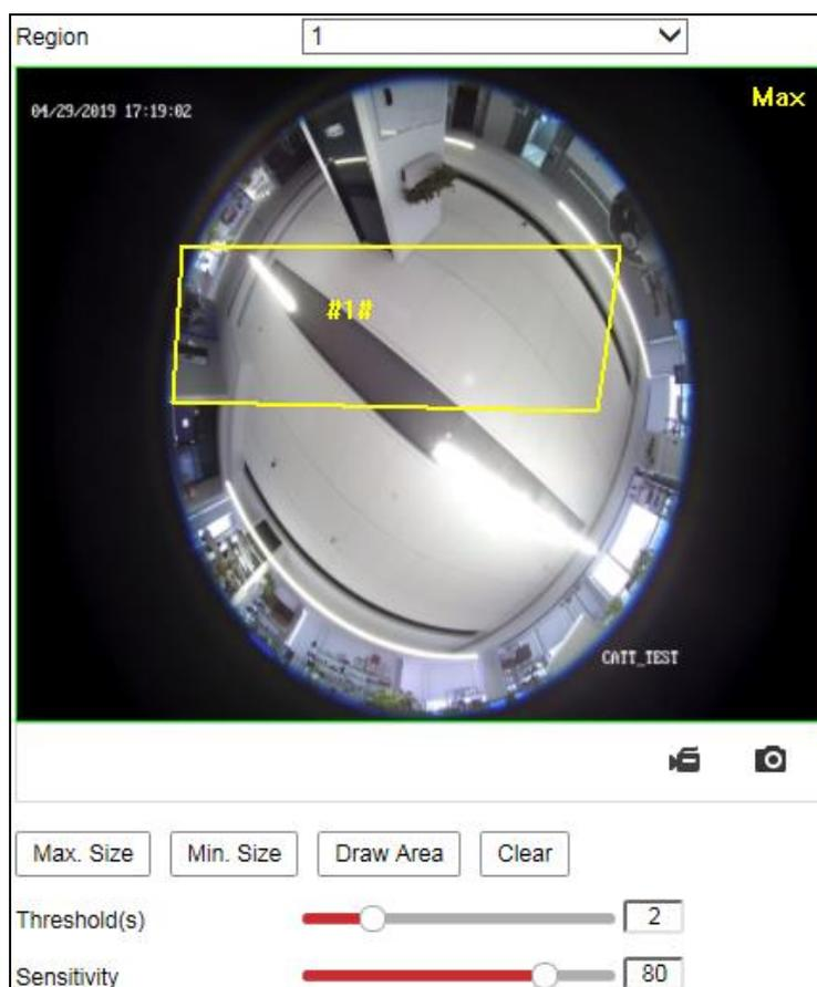
Figure 9-10 Intrusion Detection
