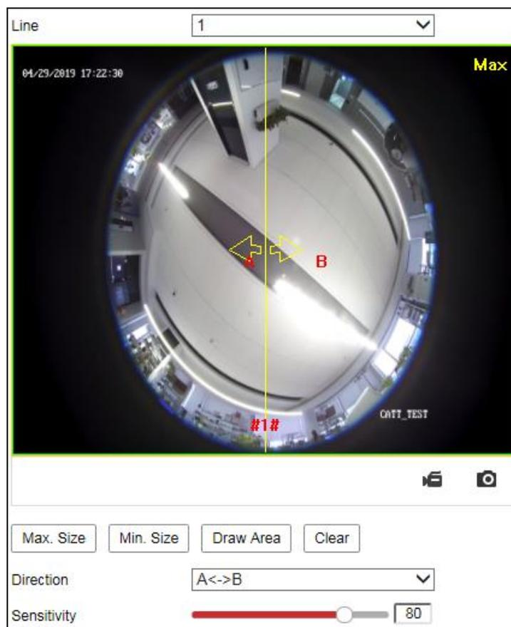
Figure 9-11 Line Crossing Detection
