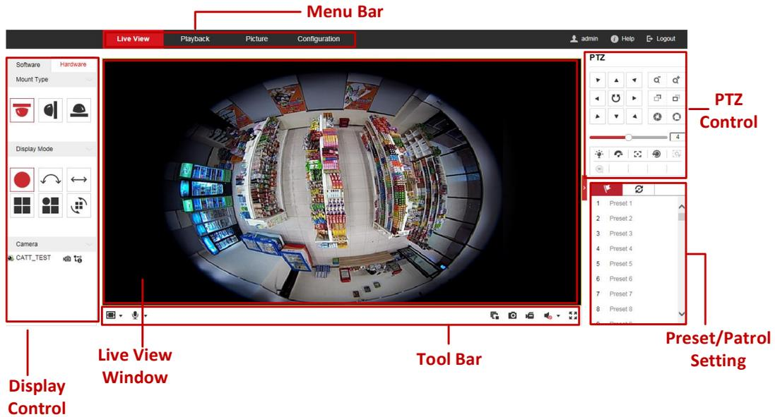
Figure 4-2 Live View Page (Hardware Decoding)
