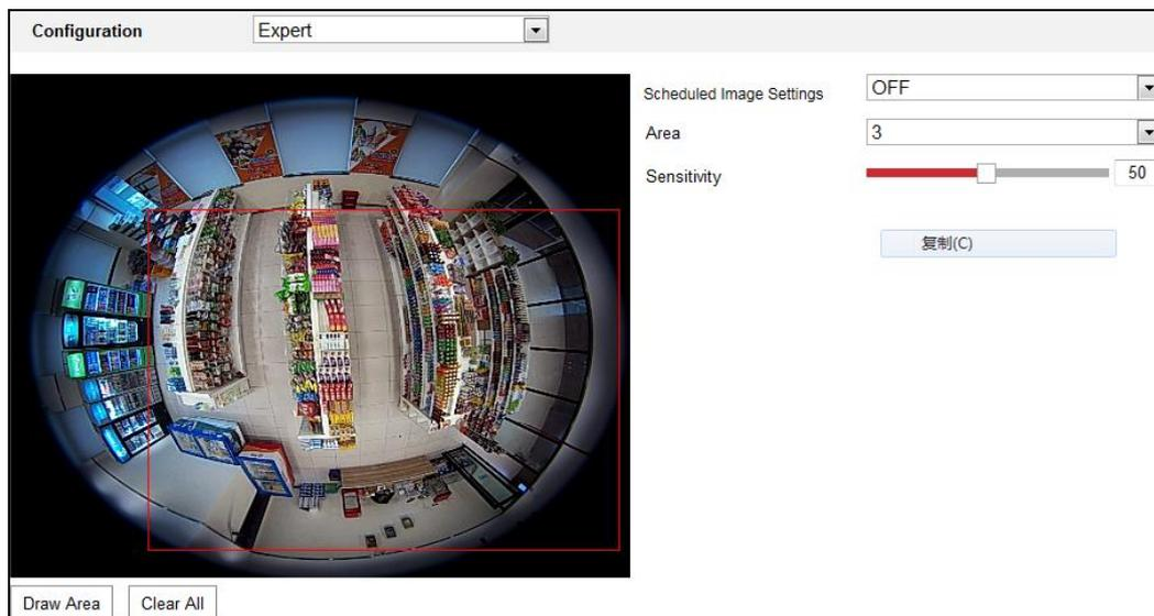
Figure 9-4 Motion Detection Settings-Expert Mode
