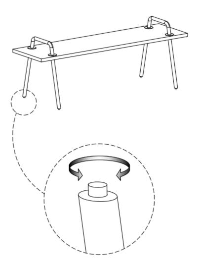
**NOTE:** Levelers on the bottom of the legs can be adjusted if floor is uneven.
