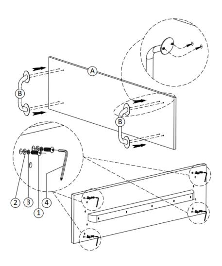
1. Use eight Allen Key Bolts 1 eight Washers 2 and eight Lock Washers 3 to attach Handrails to Top A.
