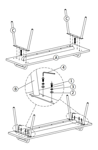
1. Use eight Allen Key Bolts 1 eight Washers 2 and eight Lock Washers 3 to attach Legs C to Top (A).
