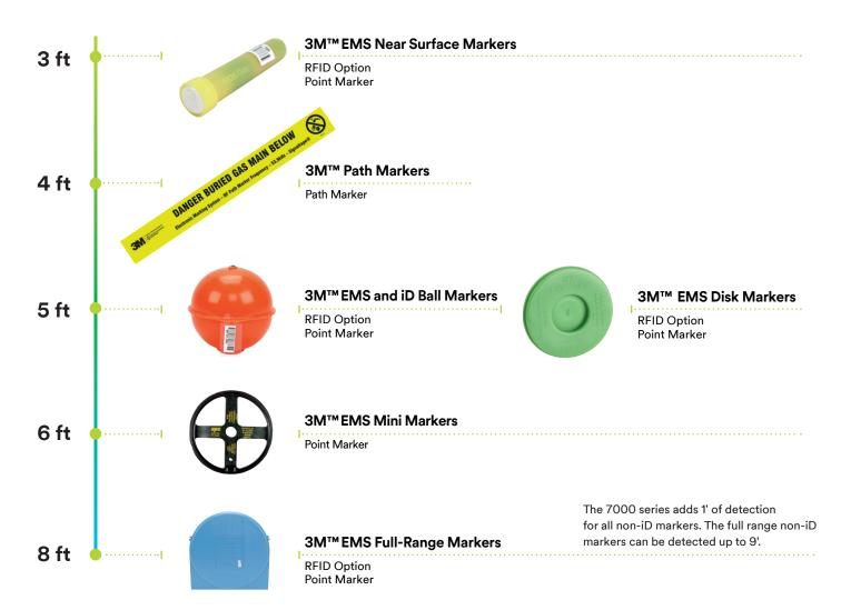
**Note:** burial depths are approximate. Review the marker specification sheet and locator compatibility for precise indication of burial depth for each of the marker models.
