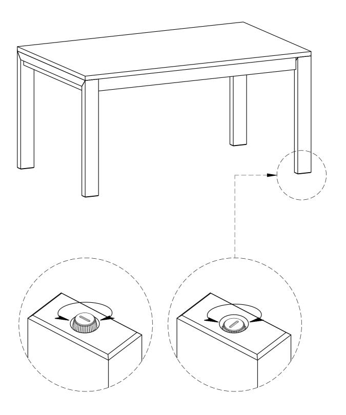
Note: Levelers on bottom of legs can be adjusted if floor is uneven.
