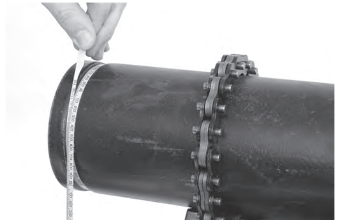
Figure 17 – Checking Groove Diameter with a Diameter Tape
