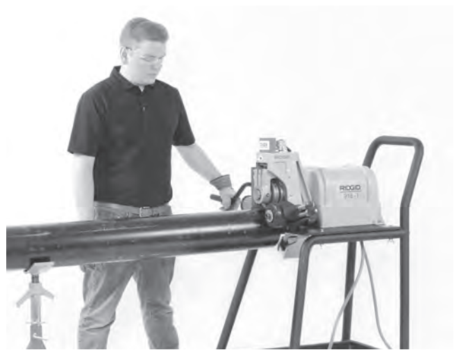
Figure 15 – Proper Operating Position
