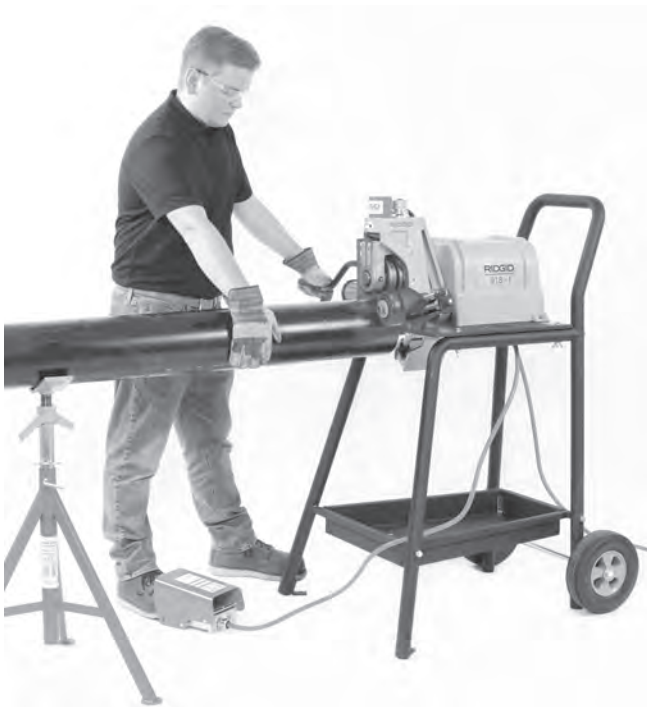
Figure 16 – Applying Pressure on Pipe
