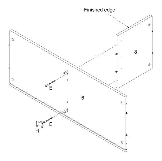
While still ensuring that the finished edge of the Cabinet Divider Board (8) is facing out, secure the Cabinet Divider Board (8) to the other side of the Shelf (6) using the (C) Cam locks. Tighten with a screwdriver!
