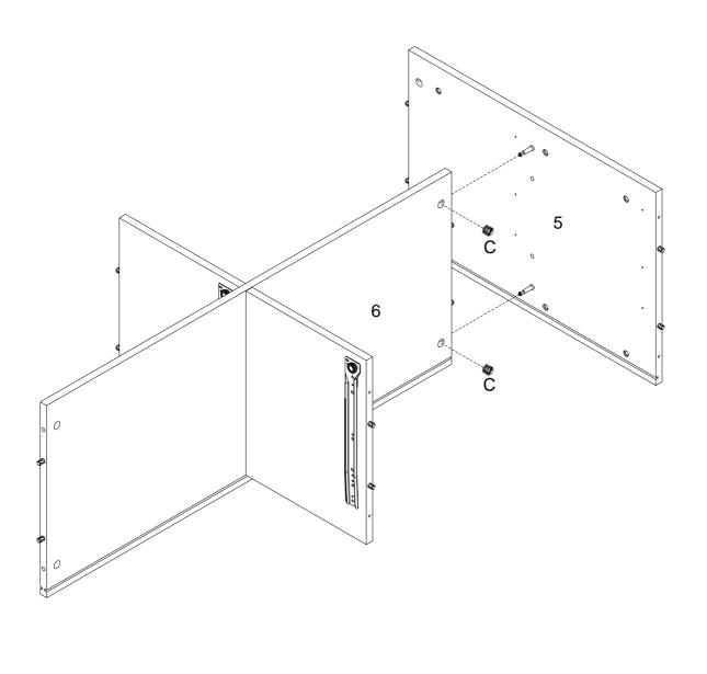
Now, repeat that for the other side! Secure the left side of the Shelf (6) to the Left Cabinet Panel (4) using the (C) Cam locks. Tighten with a screwdriver.
