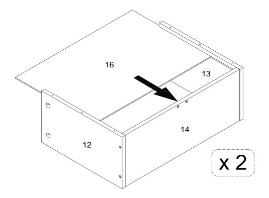
Fasten the Drawer Support (15) to the Drawer Back Panel (14) using the (J) Screws.
