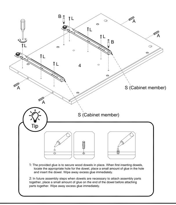
Now, follow that same process for the Cabinet Divider Boards (8)! Insert Wooden dowels (A) into the corresponding spots in the Cabinet Divider Boards (8). Screw the Cabinet member side of the (T) Drawer Glide into each Cabinet Divider Board (8) using the (L) Screws.
