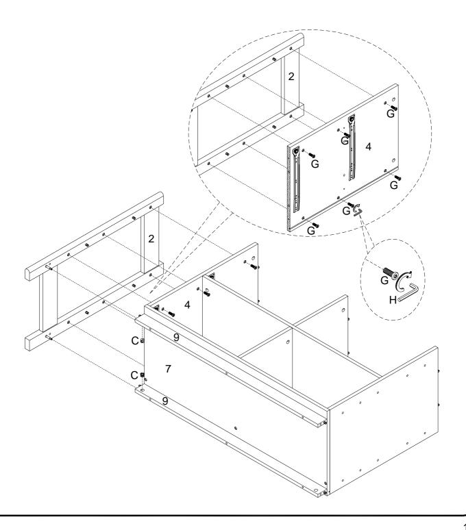
Now, repeat that process for the other side! Secure the Right Cabinet Foot Frame (3) to the right side of the unit using the (G) Bolts. Tighten with the Hex key. Make sure to also insert the Cam locks (C) and tighten with a screwdriver.
