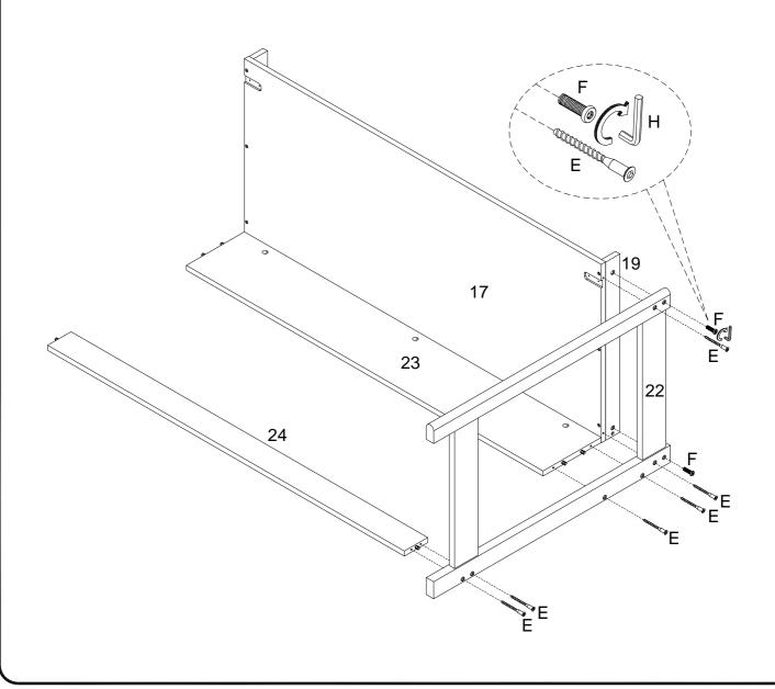
Now repeat that for the other side! Attach the Desk Bottom Trim Panel (24), the Back Desk Panel (23), and the Desktop (17) to the Left Desk Foot Frame (21) using the (F) and (E) Bolts. Tighten with the Hex key.
