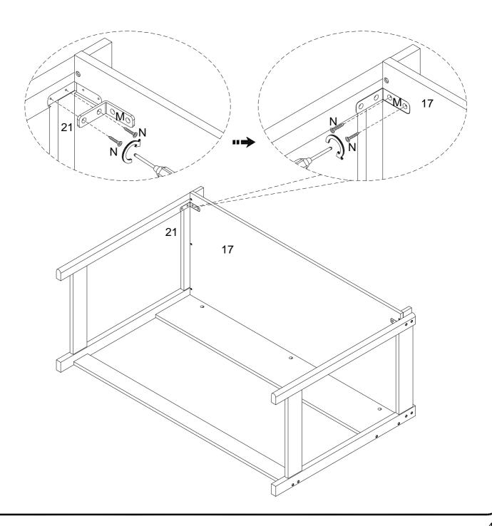
Repeat that for the other side! Secure the L-shaped bracket (M) to the Desktop (17) and the Right Desk Foot Frame (22) using the (N) Screws.
