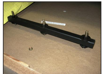
Securely fastened high quality black anodized steel Climate Adjusters, 13.5" x .75" square with 1/4" bolts and oversize washers. Five total approx. 36" apart.
