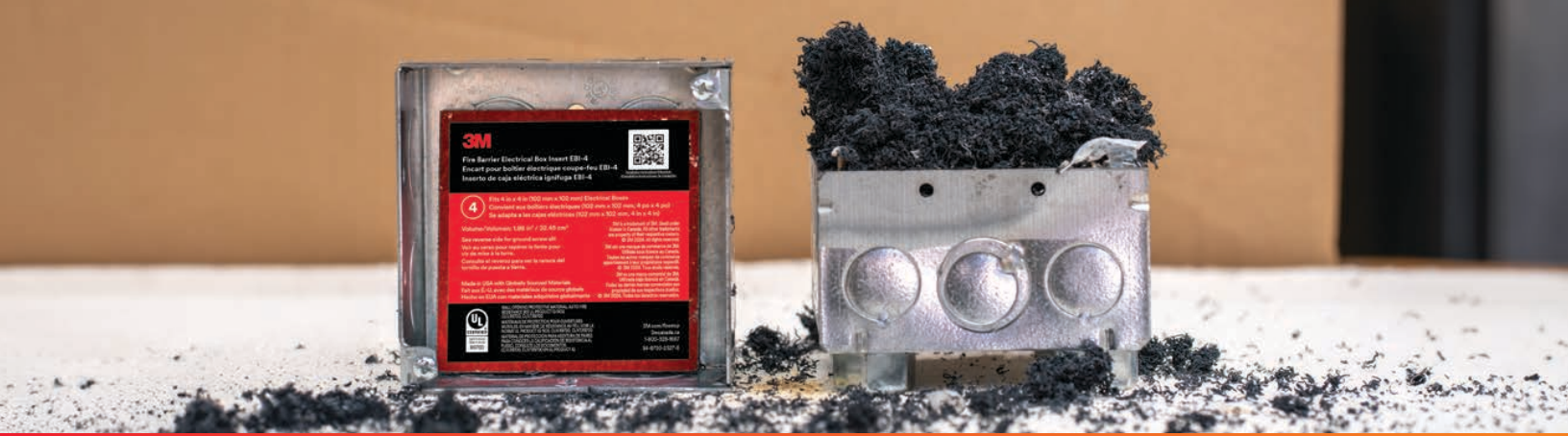
Represents Hyper-GS Intumescent Technology after fire exposure.
